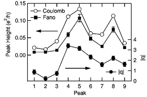
FIG. 3. Fitted  $q$  values for the peaks 1–9 in Fig. 2 are shown in the lower panel. The heights of Coulomb peaks and Fano peaks are also plotted in the upper panel. The three of them are well correlated.
