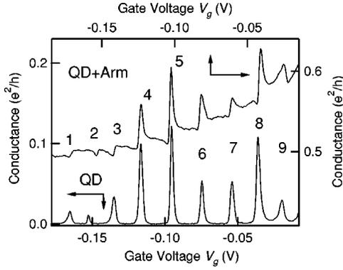
FIG. 2. Typical Coulomb oscillation at  $V_C = -0.11$  V with the arm pinched off, and asymmetric Coulomb oscillation at  $V_C = -0.085$  V with the arm transmissible. The latter shows a clear Fano effect. The Coulomb and Fano peaks are in good one-to-one correspondence as they were numbered consecutively from 1 to 9. Both of them were obtained at  $T = 30$  mK and  $B = 0.91$  T.
