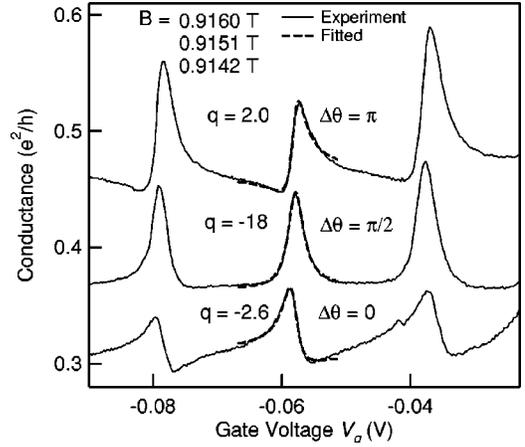
FIG. 5. Conductance of three Fano peaks at 30 mK at the selected magnetic fields at  $B=0.9142$ ,  $0.9151$ , and  $0.9160$  T. They are incrementally shifted upwards for clarity. The direction of the asymmetric tail changes between  $B=0.9142$  and  $0.9160$  T, and the symmetric shape appears at  $0.9151$  T. The results of the fitting with Fano's line shape with real  $q$ 's are superposed.
