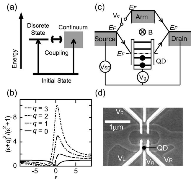
FIG. 1. (a) Principle of the Fano effect. (b) Fano's line shapes for several real  $q$  parameters. (c) Schematic representation of the experimental setup (see text). (d) Scanning electron micrograph of the correspondent device.
