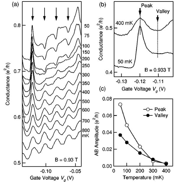
FIG. 8. (a) Conductance of the system measured between 50 mK and 800 mK at  $B = 0.93$  T. The data at  $T \leq 700$  mK are incrementally shifted upward for clarity. The Fano features marked by the arrows at 50 mK gradually disappear as the temperature increases. (b) Fano structure at 50 mK and 400 mK. (c) Temperature dependence of the AB amplitude measured at the peak and the valley indicated in (b).
