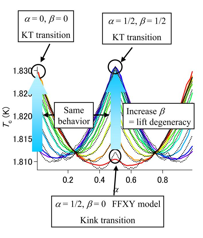
Observe the change of phase transition caused by field modulation
