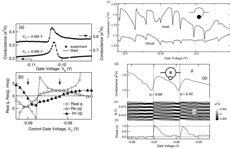
**Fig. 2:** (a) Transformation of Fano line shape by a change in control gate voltage on the reference arm. (b) Fitted values of real  $q$  and complex  $q$  in (1) as a function of  $V_C$ . (c) Temperature dependent Coulomb “dips” in conductance of a quantum wire with a side-coupled dot versus  $V_g$ . (d) Two Coulomb dips with Fano line shapes showing the same sign of  $q$ . (e) AB oscillation observed around the peaks in (d). (f) Phase shift of the AB effect in (e).
