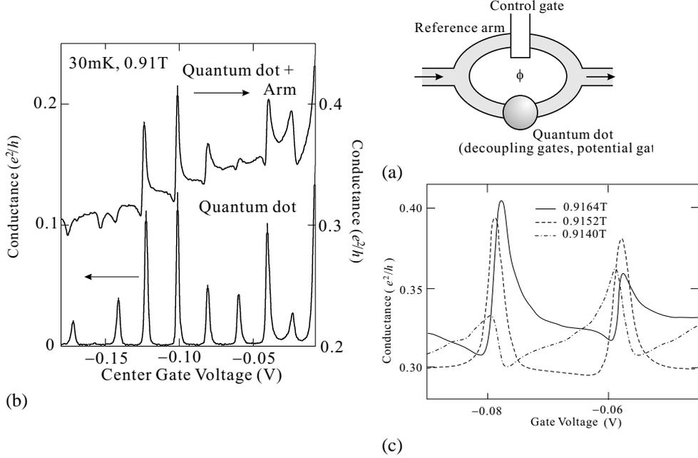
**Fig. 1:** (a) Schematic of a sample. (b) Coulomb oscillations with (upper) and without (lower) parallel conduction of reference arm. Clear Fano distortion is observed in the data with reference conduction. (c) Transformation of the Fano line shape with variation in flux piercing the ring. Broken line:  $-\phi_0/4 \equiv -(h/e)/4$ . Dotted line:  $-\phi_0/2$ .
