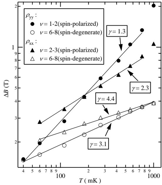
**FIGURE 2.** Width  $\Delta B$  of the magnetoresistance peaks  $\rho_{yy}$  shown in Fig.1 and  $\rho_{xx}$  after illuminated as a function of temperature  $T$ .
