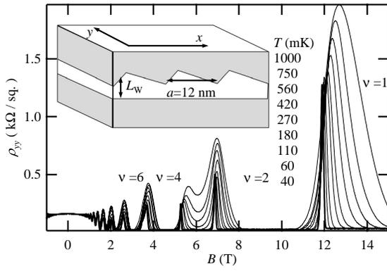
**FIGURE 1.** The insets shows the sample structure. Magnetoresistance traces of the ultrashort period LSL quantum well ( $L_w = 10$  nm, before illumination).
