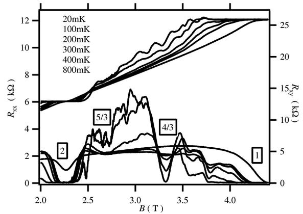
**FIGURE 2.** Magneto- and Hall resistance traces in the range of  $1 < \nu < 2$  at different temperatures.
