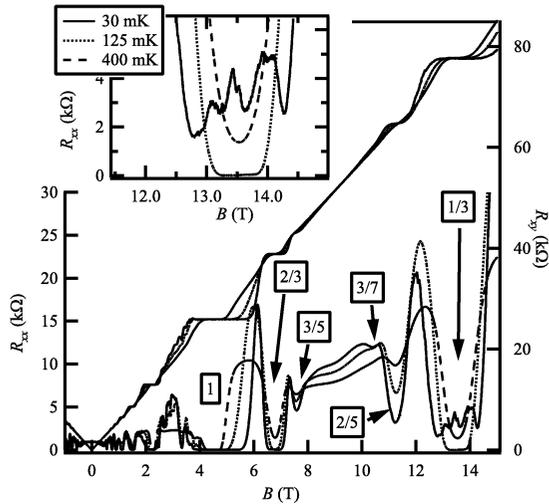
**FIGURE 1.** Magneto- and Hall resistance traces at temperatures  $T = 30, 125, 400$  mK. The inset shows the part in the vicinity of  $\nu = 1/3$  in an expanded scale.
